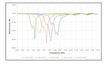
Figure 2 – Input Return Loss vs Grouped Tuning Settings
