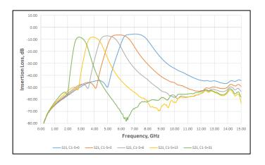
Figure 1 - Insertion Loss vs Grouped Tuning Settings
