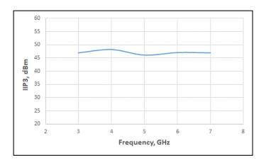
Figure 7 - In-Band IIP3 vs Frequency
