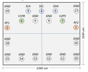
Figure 7 - Pin Configuration (Bumps Up)
