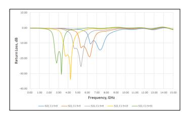
Figure 3 – Output Return Loss vs Grouped Tuning Settings
